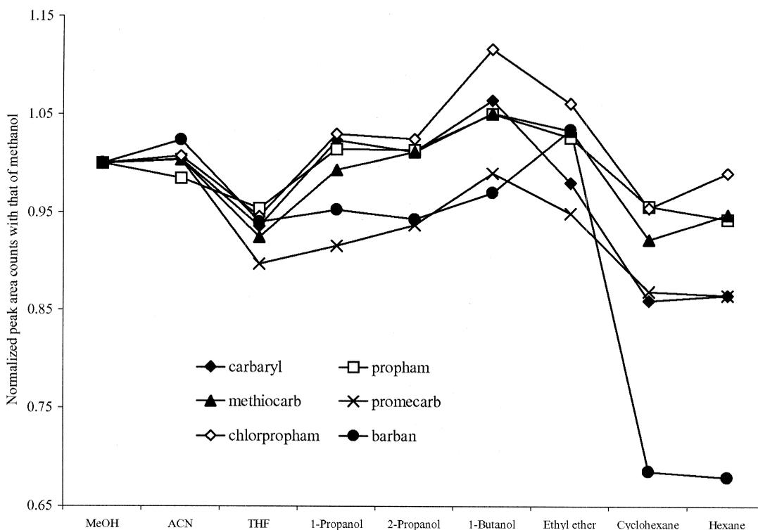
Fig. 3. Comparison of the desorption efficiencies of the solvents studied to that of methanol. Sample concentration: 2000  $\mu\text{g/l}$ , 25 a/d steps, six replicates for each solvent.
