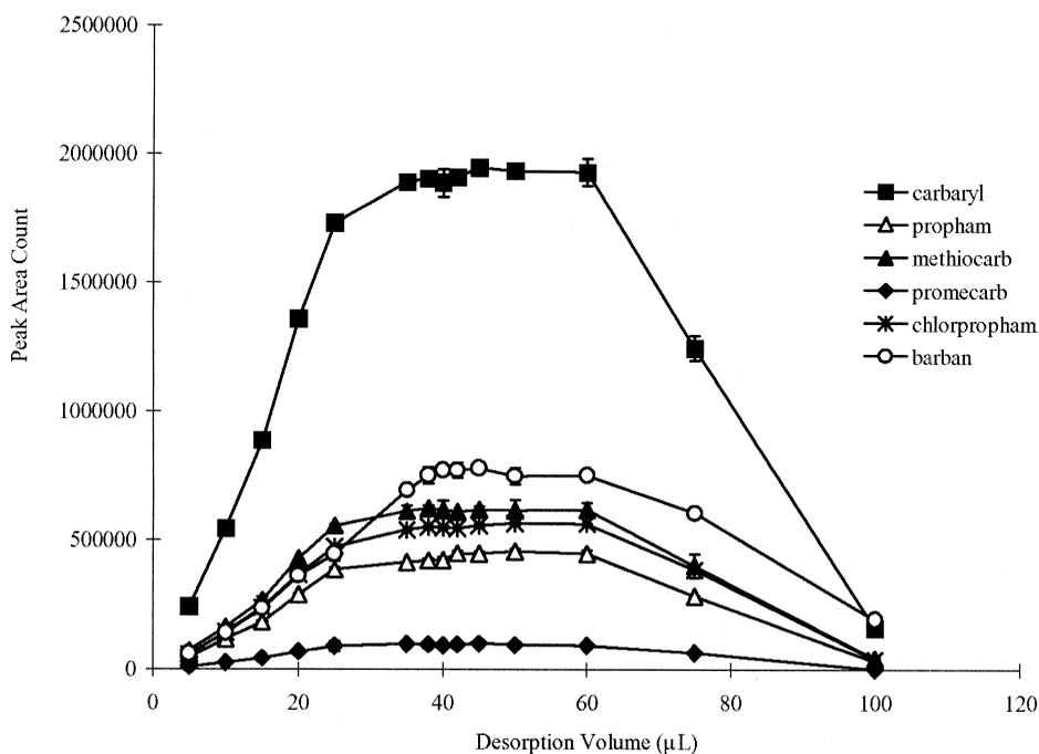
Fig. 4. Desorption curves for the carbamates studied. Sample concentration: 2000  $\mu\text{g}/\text{l}$ , 25 a/d steps,  $n=2$ . Error bars indicate the standard deviation (SD) to the mean. The absence of error bars indicates that the SD is smaller than the symbol size.
