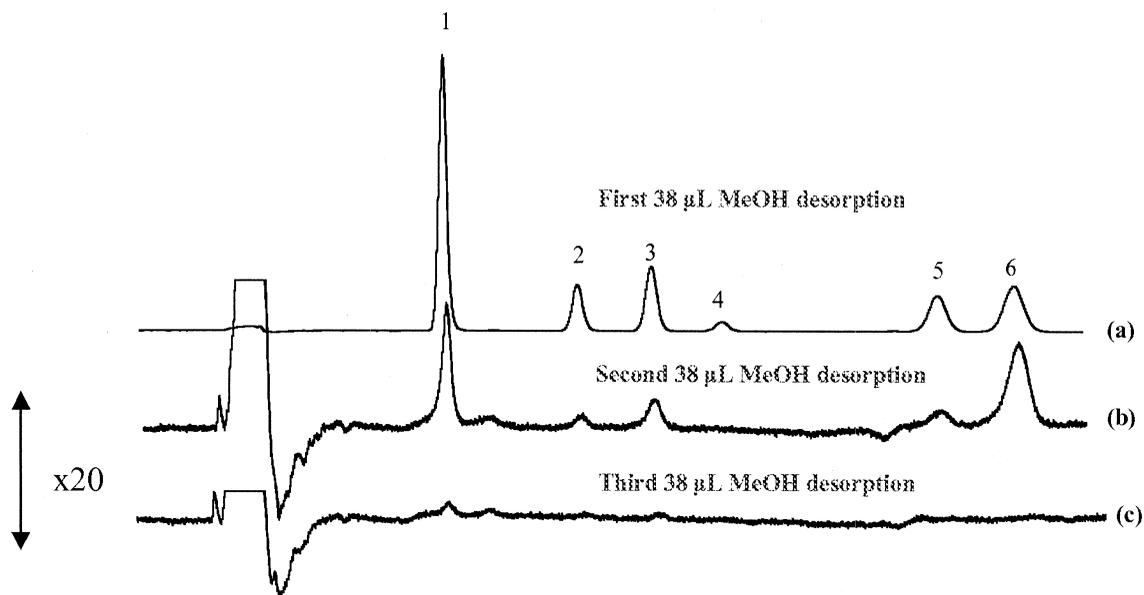
Fig. 5. Carryover study. (a) In-tube SPME–HPLC of six carbamates using 25 aspirate/dispense steps with desorption solvent of methanol 38  $\mu\text{l}$ ; (b) trace resulting after a second 38  $\mu\text{l}$  methanol desorption; (c) trace resulting after a third 38  $\mu\text{l}$  methanol desorption. Note the y-axis in the case of (b) and (c) is expanded 20 times. Peak identifications: (1) carbaryl; (2) prophan; (3) methiocarb; (4) promecarb; (5) chlorprophan; (6) barban.
