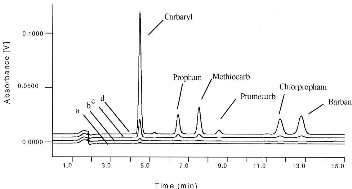
Fig. 6. Chromatograms of extraction and analysis of six carbamates using the in-tube SPME–HPLC method with four concentrations: (a) 5, (b) 10, (c) 100, and (d) 1000  $\mu\text{g}/\text{l}$ , a/d steps=15.
