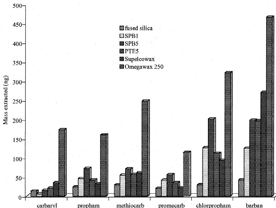
Fig. 1. Comparison of the extraction efficiencies with the different capillaries. Sample concentration: 2000  $\mu\text{g}/\text{l}$ , 25 aspirate/dispense (a/d) steps, six replicates for each capillary.
