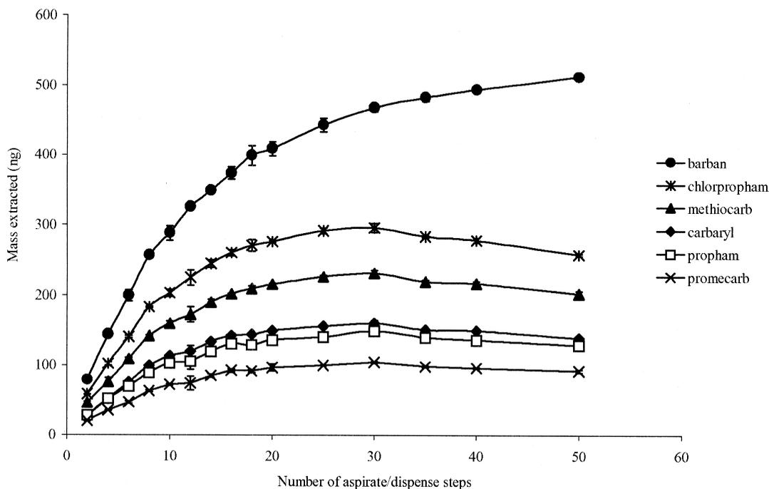
Fig. 2. Extraction profiles (number of aspirate/dispense steps) for six carbamates using a Omegawax 250 capillary. Duplicate aqueous samples were extracted using 2, 4, 6, 8, 10, 12, 14, 16, 18, 20, 25, 30, 35, 40 and 50 aspirate/dispense steps.
